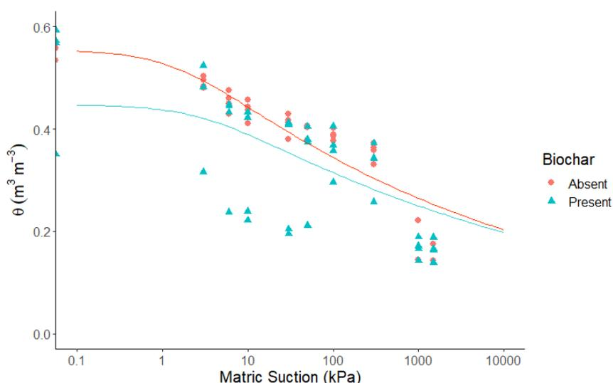
Figure 3 – Water retention curves under the absence and presence of biochar with  $N = 4$  for each matric suction. The lines are the fitted water retention and circles and triangles are the observed soil humidity.
