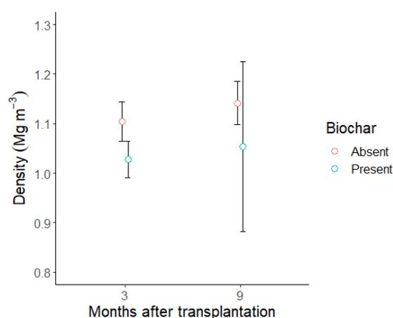
Figure 2 – Soil bulk density. Above and below bars are 95% confidence interval with N = 15 and 4 for 3 and 9 months, respectively.
